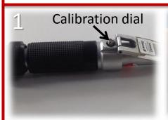
To calibrate the refractometer, firstly ensure that it is clean. Wipe the surface with a clean tissue and distilled water.
