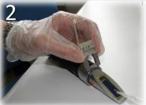
Place a small volume (one or two drops) of distilled water onto the reading surface and close the lid.
